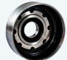
Polymer diffuser flow paths and inner polymer lining
